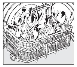
Unsorted cutlery should be placed in the cutlery basket with the handles facing downwards to ensure optimum spray water access. Mowever, to avoid the risk of injury cutlery with sharp points should be placed with the handles upwards.
